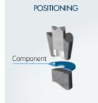
The component is positioned at the insertion position above the staking die. Component has not contact with staking die.
